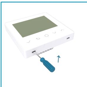
**1.** Using a small flat-blade screwdriver to insert it into the empty slot at the front cover. Then use the screwdriver to pry the thermostat forward, and then please separate the front cover from the back cover by hand carefully.
