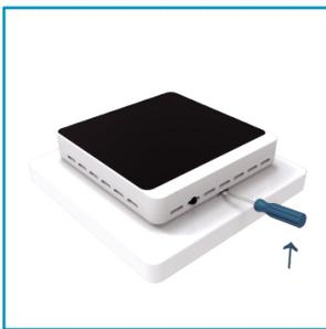
**1.** Using a small flat-blade screwdriver to insert it into the empty slot at the bottom of the middle frame that is in contact with the front cover. Then use a screwdriver to pry the thermostat forward, and then please separate the front cover from the back cover by hand carefully.
