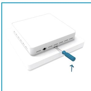
**1.** Using a small flat-blade screwdriver to insert it into the empty slot at the bottom of the cover frame that is in contact with the front cover. Then use a screwdriver to pry the thermostat forward, and then please separate the front cover from the back cover by hand carefully.
